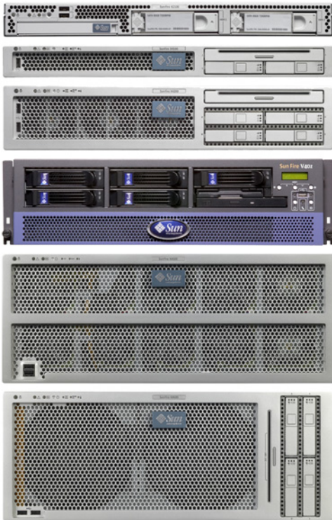
Sun Fire X2100, X4100, X4200, V40z, X4500, and X4600 servers (top to bottom)
