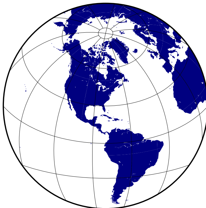
Figure 10.6: Hemisphere map using the Lambert azimuthal equal-area projection.
